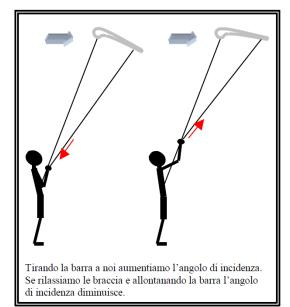
At the zenith the kite has an angle of incidence with the wind close to zero: thus it has a small power and is the ideal location if we want to spop and relax.
