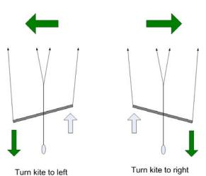
rotate (more pronounced will be the pulling of the bar, highter will be the rotation of the kite). For making practice on control of the kite, we should make rotation of the kite similar to  $\infty$  in the wind window: initially keeping the kite up and running close to the zenith, then with some wide  $\infty$ , until the edges of the wind window.
