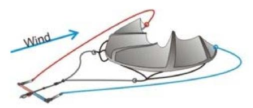
Kite with lines correctly installed
